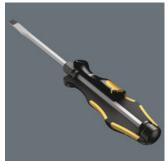
A hexagon blade made out of highquality bit material extends right through the handle - thereby ensuring full transfer of force, even when struck with a hammer. The ductile tempered material prevents the blade from splintering or breaking.
