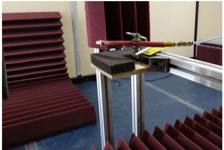
Figure 3: The hose leak type measurement at an angle of 30 degrees.
