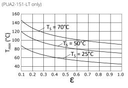
Graph showing the minimum measurable object temperature (Tmin), determined by surface emissivity ( $\epsilon$ ) and sensor temperature (TS).
