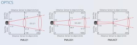
Diagrams show the diameter of the measured spot versus the distance from the lens of the sensor. The measured spot sizes shown here contain 90% of the energy the sensor detects. We normally recommend the target size should be at least twice the measured spot size for maximum accuracy. All PyroMiniUSB models will measure at longer distances than the diagrams show, with a larger measured spot size.
