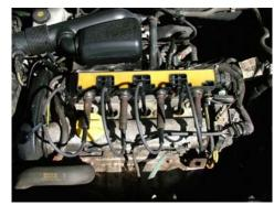
This system can only be tested if you have the same number of extension leads as coils within the cartridge coil-pack. The cartridge coil-pack is fitted directly over all the spark plugs and lifts off in one unit.
