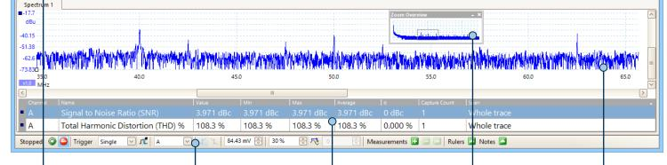
Movable axes: The vertical axes can be dragged up and down. This feature is particularly useful when one waveform is obscuring another. There's also an Auto Arrange Axes command.
