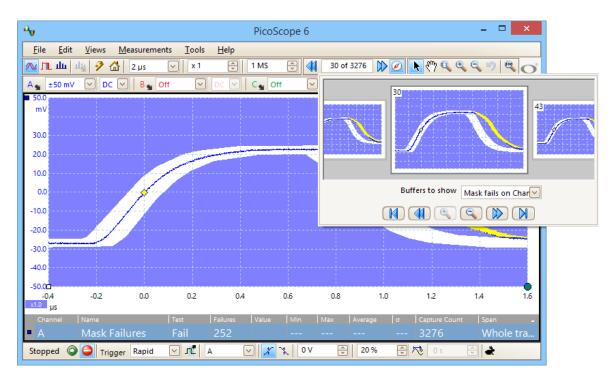
As well as simple edge triggers, a selection of time-based triggers are available for both digital and analog inputs.
