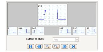
When the trace length is set to be shorter than the scope's memory, the PicoScope will automatically configure the memory as a circular buffer, recording recent waveforms for review. For example, if 1 million samples are captured, up to 500 waveforms will be stored in oscilloscope memory. Tools such as mask limit testing can then be used to scan through each waveform to identify anomalies.
