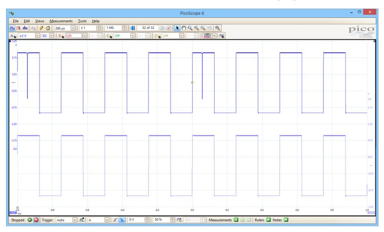
In the example above, both waveforms show the same signal using different types of hardware acceleration. The top waveform has used the aggregation possible with a PicoScope, and as a result the high-frequency spikes are preserved. The bottom waveform has used traditional decimation, showing a loss of high-frequency information.
