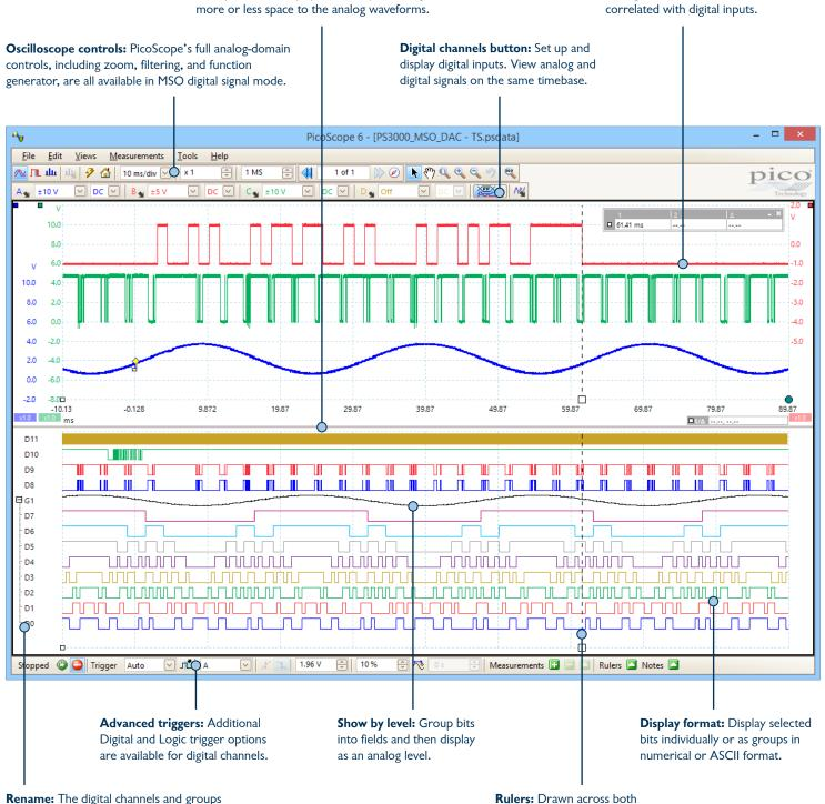
**Rename:** The digital channels and groups can be renamed. Groups can be expanded or collapsed in the digital view. **Rulers:** Drawn across both analog and digital panes so signal timings can be compared.
