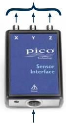
6 pin DIN plug for accelerometer connection
