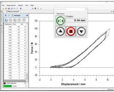
Control of the test stand using SAUTER PC software AFH
