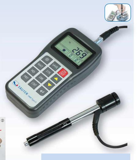
Automatic recognition of the impact sensor connected to the HMP
