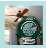
Extech's RH35 monitors Humidity, Temperature, and Dew Point for the previous 24 hours and alerts users to indoor mold hazard conditions starting with a frown icon warning when humidity reaches 60%RH. When the RH exceeds 65%, a loud audible alarm and bright flashing red LED will be triggered. The frown icon will also appear if the environment is too dry (<40%RH) where static electricity becomes a concern.
