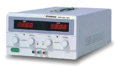
The GPR-H Series is single output, 240 to 375W, linear DC power supply Overload and reverse polarity protection keep GPR and loads safe from unexpected conditions. High regulation and low ripple/noise are maintained at 0.01% and less than 1mVrms, respectively. Internal load selection, continuous or dynamic, accommodates applications such as pulsed current. The GPR-H Series is suitable for middleto high-end bench-top application requiring preciseness.
