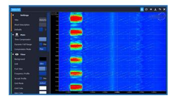
Spectrogram / Waterfall View for the identification of frequency hops, measurements of pulse rate, analysis of time variant spectra and the tuning of a VCO
