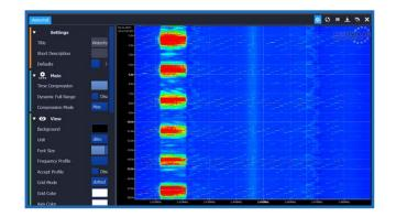
Spectrogram / Waterfall View for the identification of frequency hops, measurements of pulse rate, analysis of time variant spectra and the tuning of a VCO
