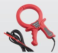
SC-600-EUR Signal Clamp The Signal Clamp accessory provides an efficient and safe method of applying a locate signal to a cable, enabling the Transmitter to induce a signal through the insulation into the wires or pipes. The clamp works on low impedance closed circuits only.
